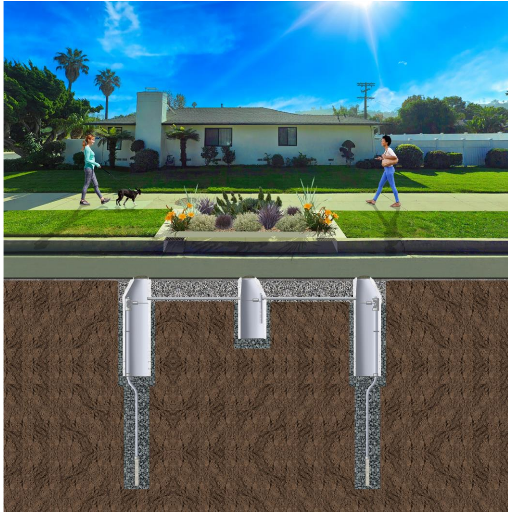
Parkway Bioswales and Drywells
