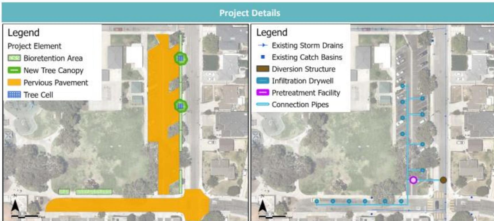
**Figure 1. Surface (Left) and Subsurface (Right) Project Site Layout**
