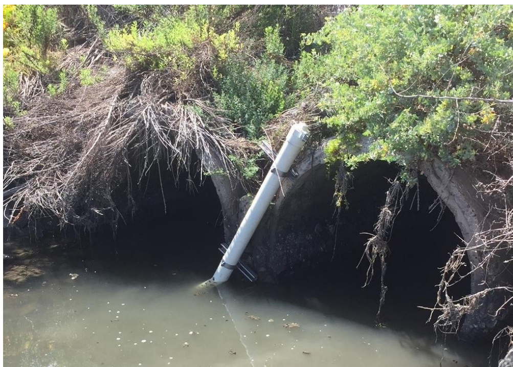
Figure 13. Common Installation of a Long-Term Data Sonde in an Open Water Body
