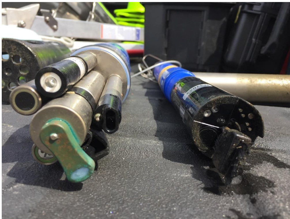
Figure 12. Sensors Installed on Two Different Manufacturer Multi-Parameter Data Sondes
