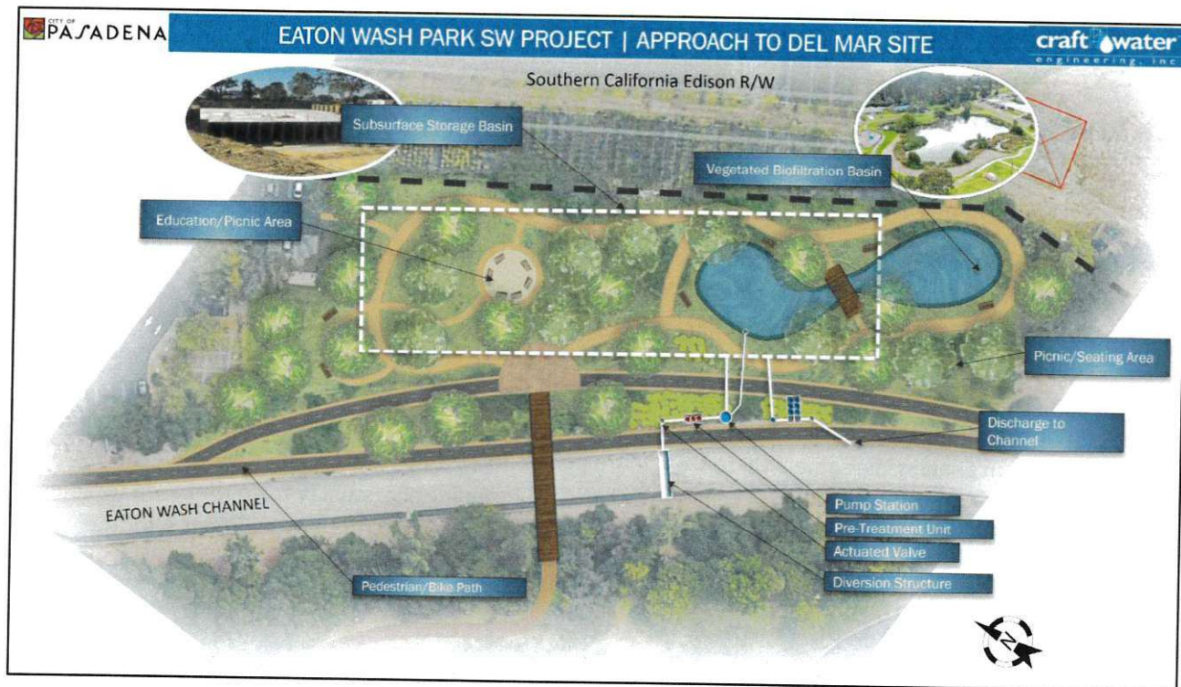
Figure 4-3. Del Mar Site Utility Concept Plan
