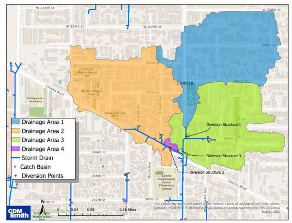
Figure E-1. Drainage Areas and Proposed Diversions
