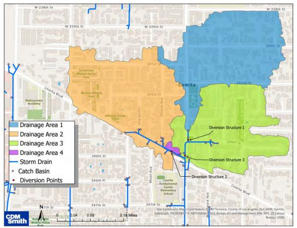
Figure 2-2. Existing LACFCD Storm Drains and Tributary Areas
