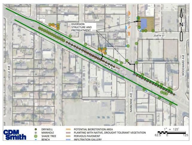
Figure 1 – Original Concept Design Layout
