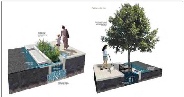
Figure 2-6. Typical Bioretention and Tree Well (Source: Philadelphia Green Streets Design Manual)
