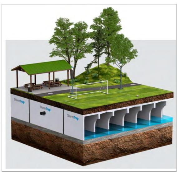
gallery should be a minimum 3,100 SF to manage the entire design storm. Final sizing will be refined during the design phase.
