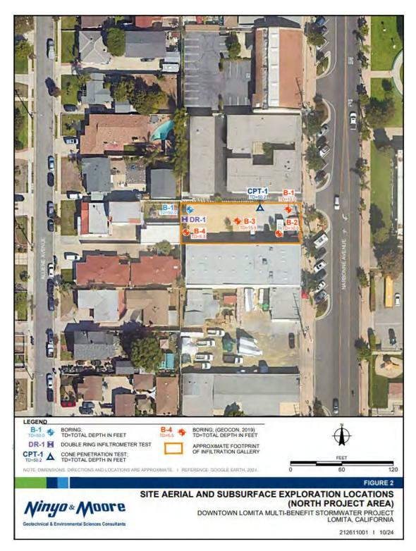
Figure 2 – Geotechnical Investigation Near Proposed Infiltration Gallery
