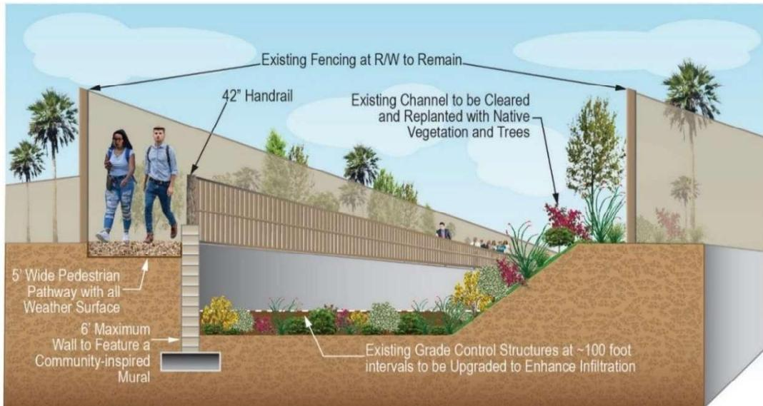
Figure 2 Conceptual Typical Cross-Section of Project's Channel Improvements (Looking Upstream)
