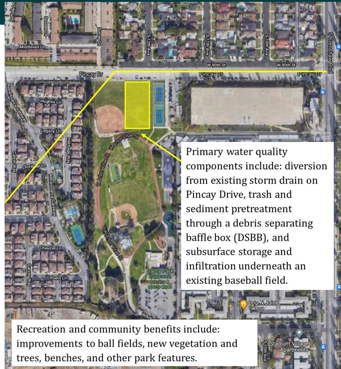
Primary water quality components include: diversion from existing storm drain on Pineay Drive, trash and sediment pretreatment through a debris separating baffle box (DSBB), and subsurface storage and infiltration underneath an existing baseball field.
