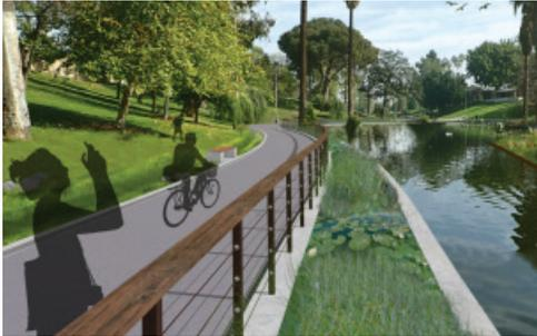
‘Green stormwater infrastructure’ involves decentralized stormwater management practices, such as green roofs, trees, rain gardens, and permeable pavement that can capture and infiltrate rain where it falls, thus reducing stormwater runoff and improving the health of surrounding waterways. Nature-based green stormwater infrastructure projects can capture and clean more stormwater while providing environmental, recreational, economic and health benefits to communities.
